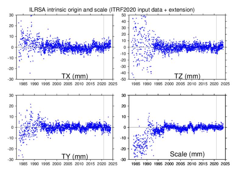
SLR Origin & scale accuracy at 2015.0 below 1 mm and scale stability at the level of 0.1 mm/yr
