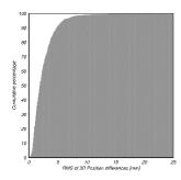
92% of the weekly 3D differences are smaller than 5 mm. Largest differences are located at Lifou and Iquique, sites with very short time spans and for which we did not estimate periodic terms in version 3.0 as the sites were turned off before mid-2002.
