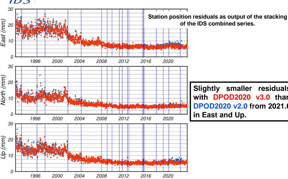
Slightly smaller residuals with DPOD2020 v3.0 than **DPOD2020 v2.0 from 2021.0** in East and Up.
