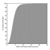
78% of the weekly 3D differences are smaller than 5 mm. Largest differences are located at Canberra, Lifou, Iquique, sites with very short time spans and for which we did not estimate periodic terms in version 3.0 as the sites were turned off before mid-2002.
