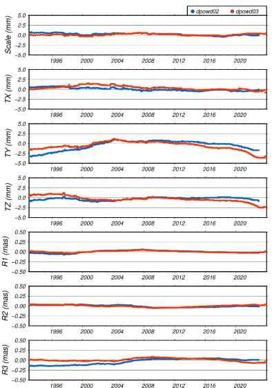
Helmert parameters of the weekly propagations of DPOD2020 version 3.0 and version 2.0 wrt ITRF2020 without annual and semi-annual corrections.
